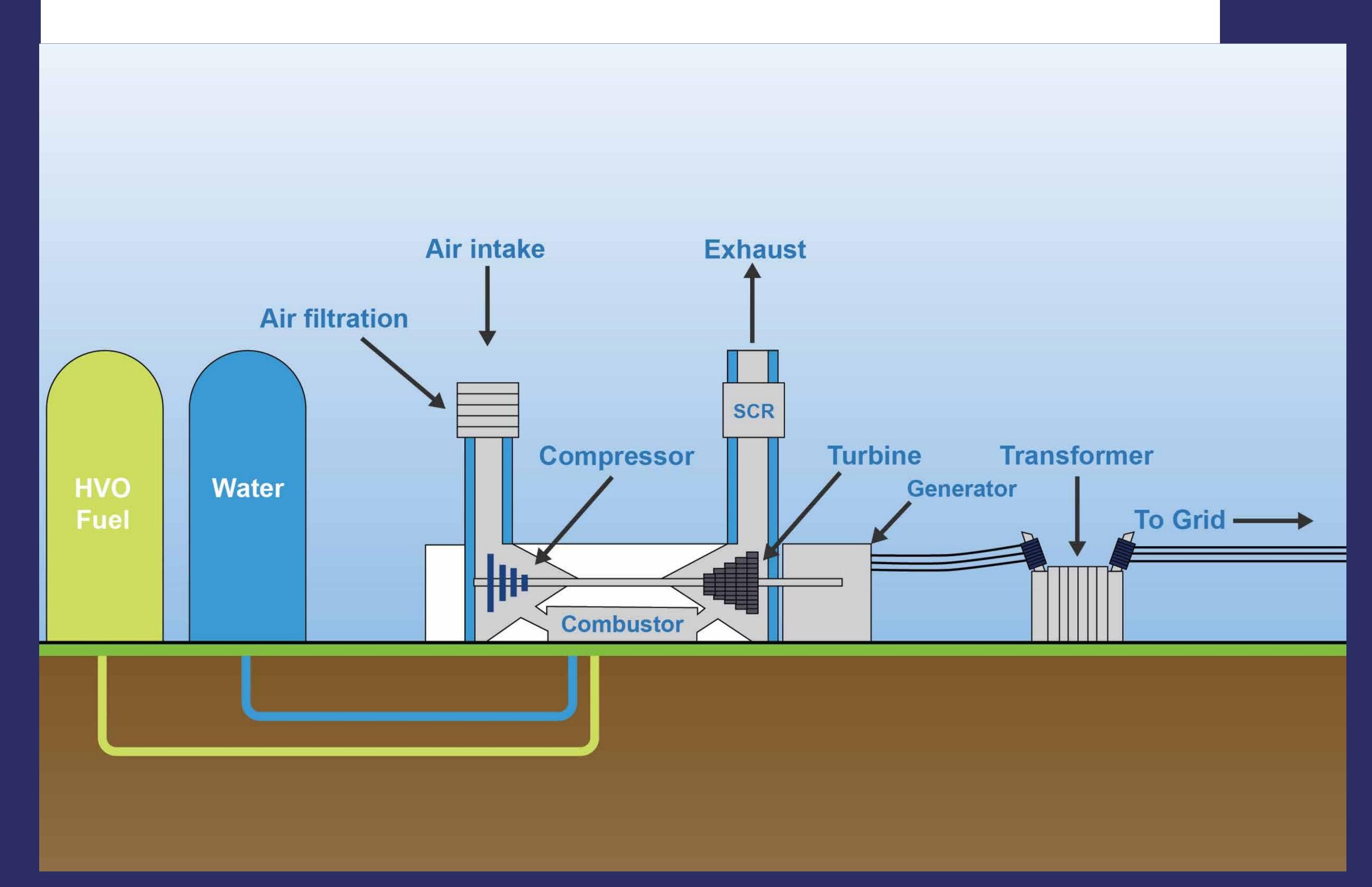
**Note:** The above visual outlines a simplified version of how an Open Cycle Gas Turbine (OCGT) power station operates.
